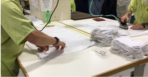
Part of the process for making masks involves attaching draw strings and ironing them to the fabric.
